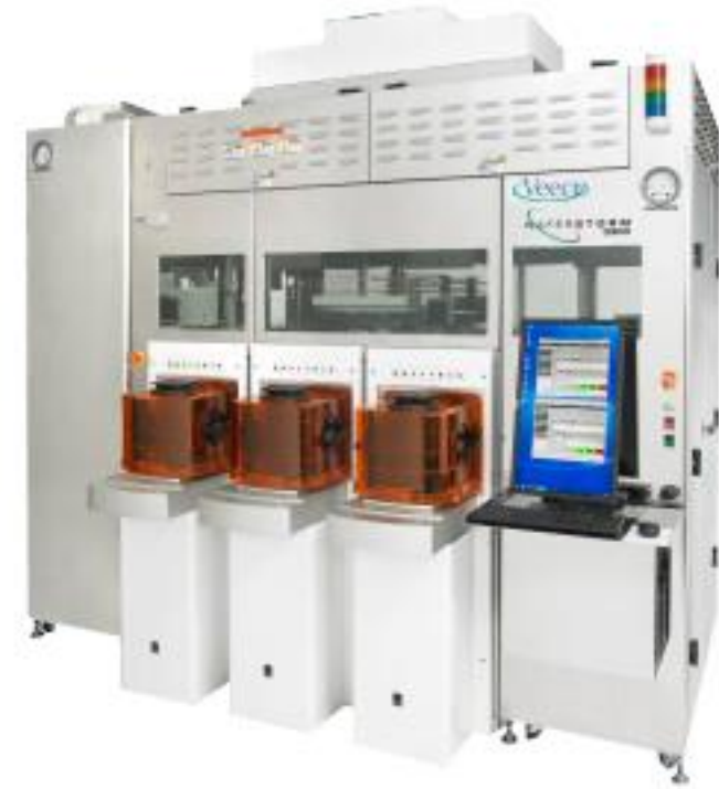
Wet/Dry etching tool (Etching+ Implant+ planarization)
